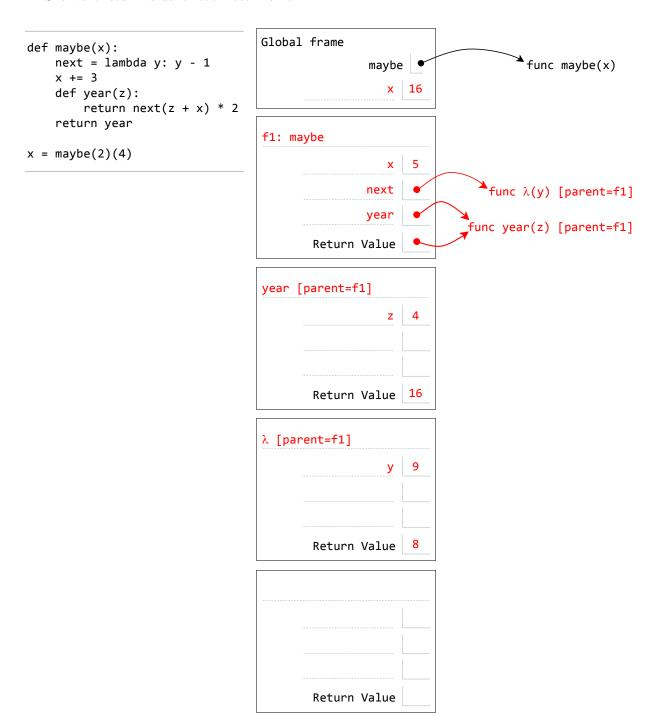
(b) (6 pt) Fill in the environment diagram that results from executing the code below until the entire program is finished, an error occurs, or all frames are filled. You need only show the final state of each frame. You may not need to use all of the spaces or frames.
