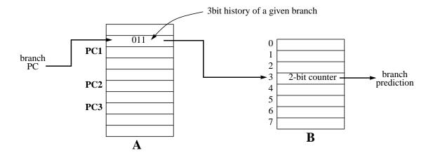
Table A is indexed by the program counter. Table B contains two-bit saturating up-down counters as described in class; they predict taken when the counter value is 2 or 3. You can assume that **PC1**, **PC2**, and **PC3** map to the *distinct* slots in the table shown above.
