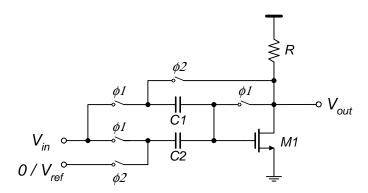
a) If the open-loop gain of the amplifier formed by M1 and R is -A, derive a closedform expression for the output residue voltage *Vout* in terms of *Vin*, *Vref*, and comparator decision D (you may assume *Vgs* of M1 is 1V when  $\phi l$  is closed). [20] *Hint: Note the quiescent biasing point of the amplifier is that when*  $\phi l$  *is closed. The open-loop gain is defined in terms of the signal swing where quiescent biasing is removed.*
