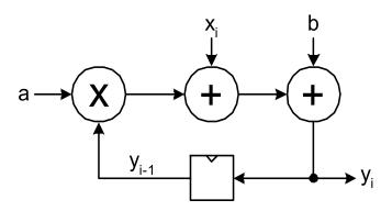
Reorder to shorten the feedback loop and try putting register after multiply:
