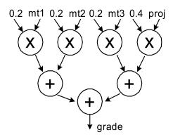
This time-multiplexing performs the action of each node one at a time. (Sort of emulates the graph it.)
