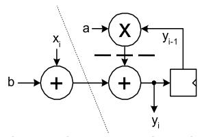
Interleaving makes operations in adjacent pipeline stages independent and allows full cycle for each:
