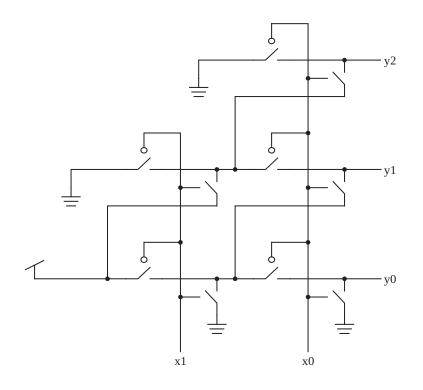
Here, switches are transmission gates as shown below.
