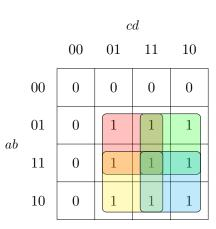
This gives us the SOP expression  $x = a \cdot c + a \cdot d + b \cdot c + b \cdot d$ . We need four 2-input AND gates and one 4-input OR gate to directly implement this. Converting the 4-input OR gate into three 2-input OR gate, seven 2-input gates are needed.
