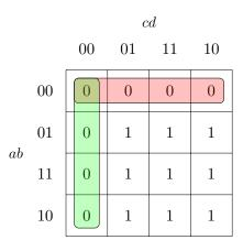
This gives us the POS expression  $x = (a + b) \cdot (c + d)$ . The direct implementation of this POS uses only two OR gates and one AND gate. Therefore, it requires only three 2-input gates.
