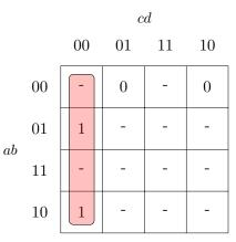
For y,the minimul SOP is  $\overline{b} \cdot \overline{c}$  derived from the following grouping.
