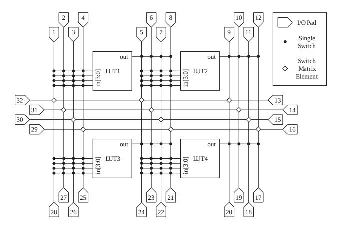
(a) What is the minimum number of switches needed to connect the output of LUT4 to the input of LUT1. (*Hint*: We need at least three switches to connect the output of LUT1 to the input of LUT4)
