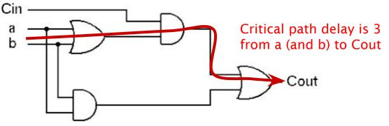
What is critical path delay in this circuit?
