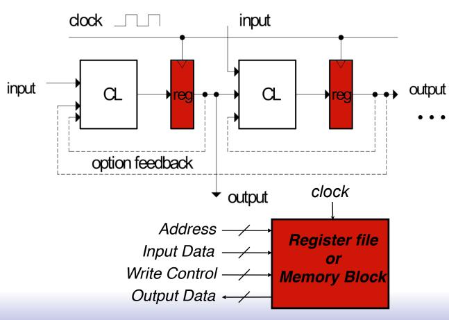
State elements are mixed in with CL blocks to control the flow of data.
