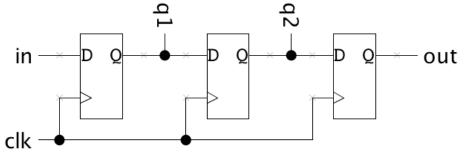
Will nonblocking and blocking assignments both produce the desired result?
