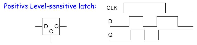
When CLK is high, latch is transparent, when clk is low, latch retains previous value.
