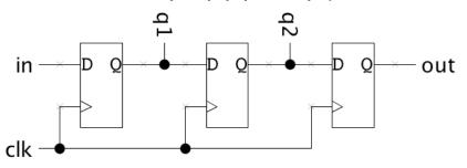
"At each rising clock edge, q1 = in. After that, q2 = q1. After that, out = q2. Therefore out = in." in --- D Q - out
