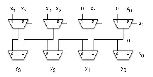
However, this places two transmission gates between the inputs and the outputs, adding unnecessary delay.
