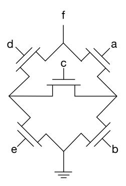
The simplest way to derive the PDN from the PUN is to find the Euler path (which is similar to finding the dual of a graph representing either network, but with the outer space split into two), as below. For more information see Rabaey, Chandrakasan, Nikolic *Digital Integrated Circuits, A Design Perspective*, Second Edition, Design Methodology Insert D.
