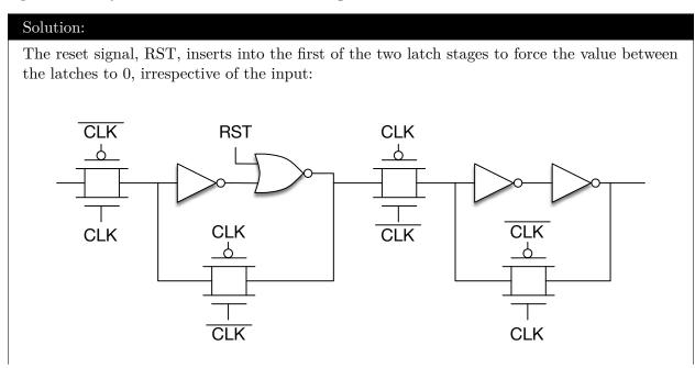
An alternative solution is to use the input multiplexor shown in the solution problem 7, but with RST used as the select input and the RST = 1 input tied to 0.
