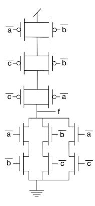
To reduce the number of gates used, factor out of one the terms in the first expression f = ab + bc + ac = ab + c(b + a). This makes it easy to deduce the PUN. Deriving the PDN from scratch is a little more work:
