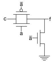
An alternative way to construct this is as a 2-1 multiplexor with one input constant and the other c, where a becomes the selection signal (or vice versa).
