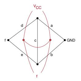
(b) From the PUN, read off the paths that result in f HIGH. Since the inputs to the PMOS transistors need to be LOW to turn them on, we treat the inputs as inverted:
