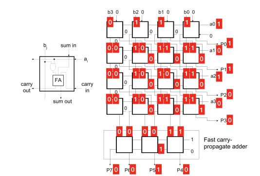
as in the figure we have for the CPA in lecture (above). Using the scheme drawn, the bits are ready in the same order as with the CPA above.
