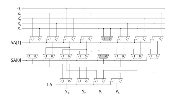
The next version uses 3 MUXs which are constructed out of 2 MUXs. The advantage of this
