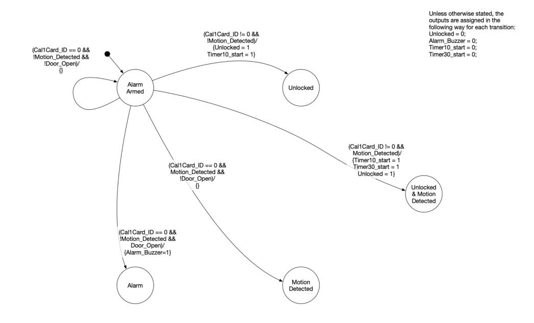
Unless otherwise stated, the outputs are assigned in the following way for each transition: Unlocked = 0; Alarm\_Buzzer = 0; Timer10\_start = 0; Timer30\_start = 0;
