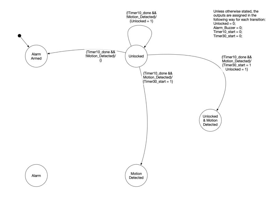
Unless otherwise stated, the outputs are assigned in the following way for each transition: Unlocked = 0; Alarm\_Buzzer = 0; Timer10\_start = 0; Timer30\_start = 0;
