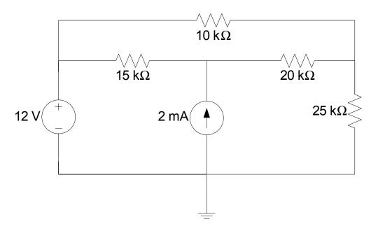
Use nodal analysis (by hand) to find the voltage at each node with respect to ground. This goes into your lab report.
