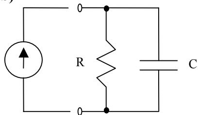
**3.** An RC (resistor + capacitor) circuit will have an exponential voltage response of the form  $v(t) = A + B e^{-t/RC}$  where A and B are constants that express the final voltage and the difference between the initial voltage and the final voltage, respectively.
