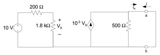
By shorting the terminals, we have changed the circuit. We cannot assume that the voltage and current values found in the  $V_{TH}$  calculation are still the same.
