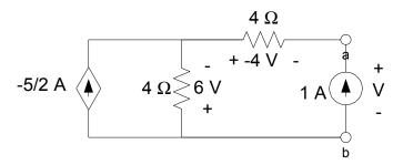
By Ohm's law, there is a 6 V drop as shown. V can now be determined using KVL (clockwise, starting at a):
