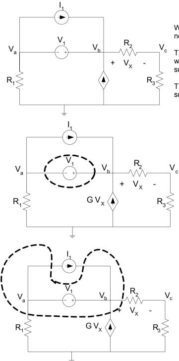
We now try to write KCL equations at each node with unknown node voltage.
