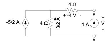
By KCL, the current flowing up the equivalent resistor must be 3/2 A.
