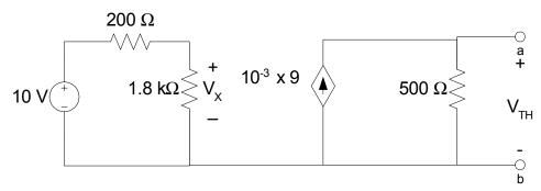
The 9 mA current flows down through the resistor. By Ohm's law, the voltage drop is 4.5 V.
