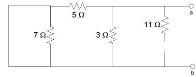
The 7  $\Omega$  resistor is shorted out, so it cannot carry nonzero voltage. The 11  $\Omega$  resistor is disconnected, so it cannot carry current. Neither have an impact on the circuit.
