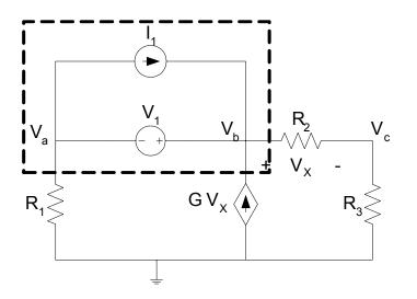
Here, the supernode is drawn around the current source as well. Anything that is in parallel with the floating voltage source can be included in the supernode.
