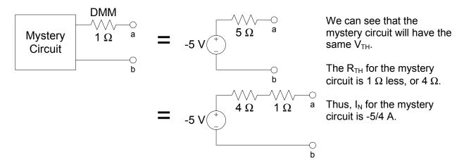
You could also solve this problem by replacing the mystery circuit with its Thevenin equivalent, with  $V_{TH}$  and  $R_{TH}$  left as unknowns. Writing KVL for the circuit with the source at 0 V, then again with the source at 10 V, will leave two equations in two unknowns and you can solve for  $V_{TH}$ ,  $R_{TH}$ , and  $I_N$ .
