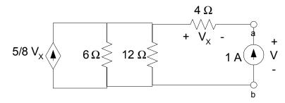
Here, a 1 A test current has been applied. We need to find V.
