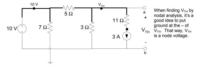
To do a shortcut, we can skip the KCL equation for the node between the 11  $\Omega$  resistor and the 3 A source. We know 3 A goes in and 3 A comes out, so 3 A goes down the 11  $\Omega$  resistor.
