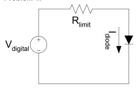
Suppose I have a voltage, V<sub>digital</sub>, that is the output of some digital circuit.
