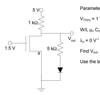
Parameters for the NMOS transistor shown are:
