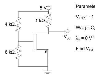
Parameters for the NMOS transistor shown are:
