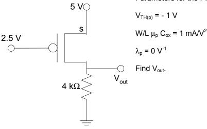
Parameters for the PMOS transistor shown are:
