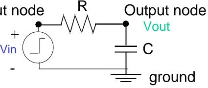
4) Solve the dc problem for the capacitor voltage after the transient is over. This is the asymptotic value.
