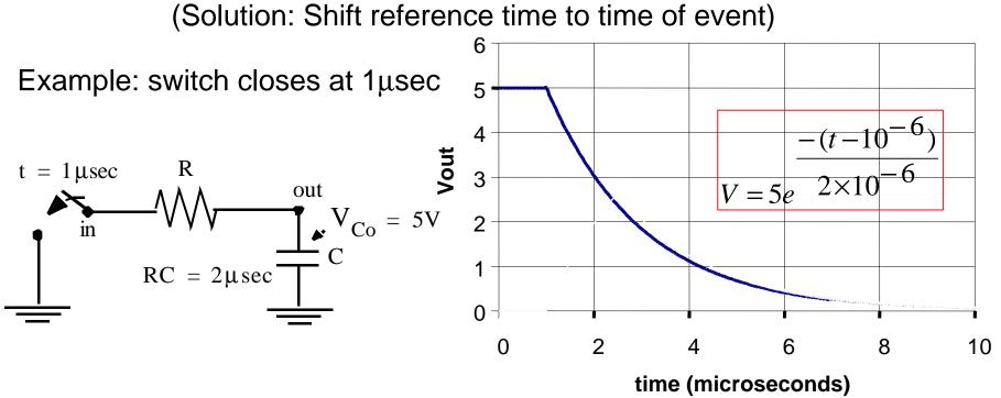
We shift the time axis here by one microsecond, i.e. imagine a new time coordinate  $t^* = t-1\mu$ sec so that in the new time domain, the event happens at  $t^* = 0$ and our standard solution applies. Of course we replace  $t^*$  by  $t -1\mu$ sec in the equations and plots. Thus instead of  $t^* = 0$  we have  $t = 1\mu$ sec, etc.
