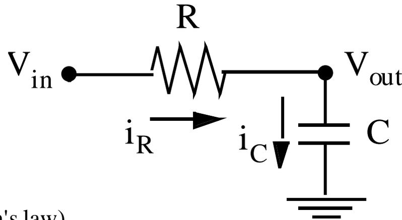
$$i_R = \frac{V_{\text{in}} - V_{\text{out}}}{R} \quad (\text{Ohm's law})$$
