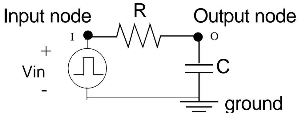
A pulse originating at **node I** will arrive delayed and distorted at **node O** because it takes time to charge  $C$  through  $R$
