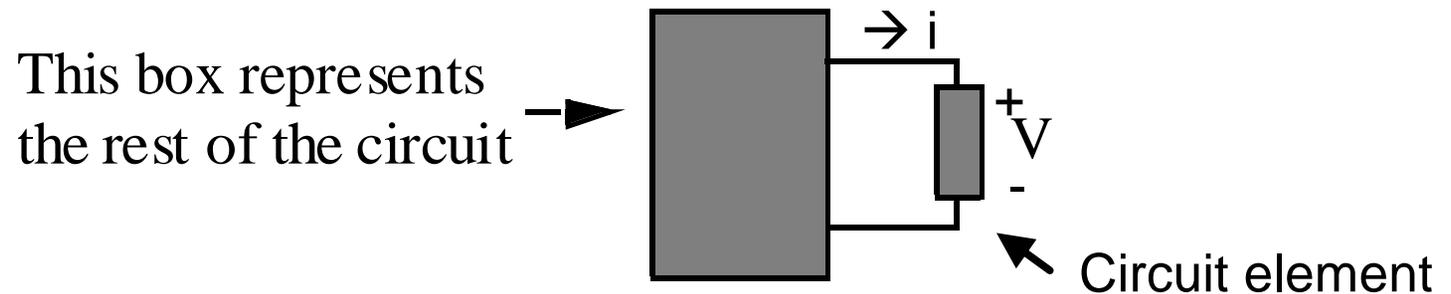
For positive current and positive voltage, positive charge “falls down” a potential “drop” in moving through the circuit element: it *absorbs* power
