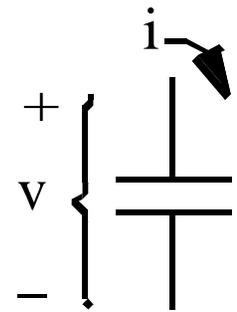
but  $dq = C \, dv$ . (We are using small  $q$  instead of  $Q$  to remind us that it is time varying. Most texts use  $Q$ .)
