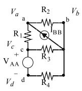
a) (5 pts.) Six nodes are shown. Determine the nodes that have potentially different voltages and assign only these nodes a label a, b, c... and voltage  $V_a, V_b, V_c...$
