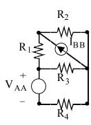
a) (5 pts.) Six nodes are shown. Determine the nodes that have potentially different voltages and assign only these nodes a label a, b, c... and voltage  $V_a, V_b, V_c...$
