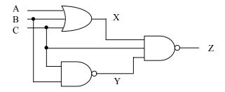
a) (9 points) Using the inputs in the diagram, determine the initial and final values of X, Y, Z.
