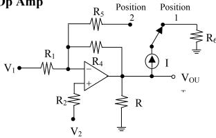
a) (10 points) Find  $V_{OUT}$  in terms of  $V_1$ ,  $V_2$ , and I, and the resistors  $R_1$ ,  $R_2$ ,  $R_3$ ,  $R_4$ ,  $R_5$ ,  $R_6$  when the switch is in position 1.
