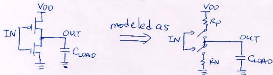
If  $R_P = 1.5k\Omega$ ,  $R_N = 1.0k\Omega$ ,  $C_{Load} = 1\text{pF}$ , what is the delay from IN to OUT when OUT is making a low to high transition? A High to low transition? What is the average?
