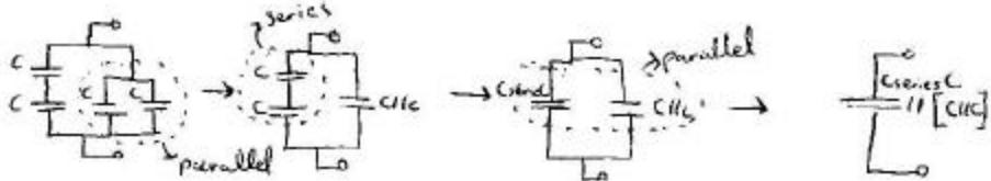
$$C_{parallel} = C + C = 4\mu\text{F}$$
