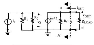
$$\frac{i_{OUT}}{i_s} = \frac{\left(R_1 \parallel R_2\right)\left(R_{OUT} \parallel R_L\right)}{R_L}$$
