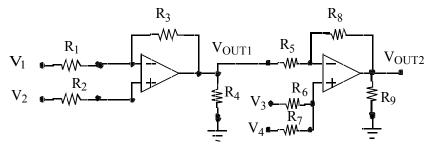
b) (9 Points) Give sufficient additional equations for finding  $V_{OUT2}$  in terms of the resistances and input voltages. Do not solve.
