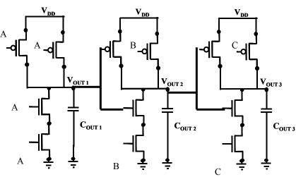
d) (8 Points) For the CMOS circuit implementation to the right of the NAND gate logic circuit above and the signal changes in part a), **find the time at which the change reaches V**<sub>OUT 3</sub>. State the delay in terms of combinations of 0.69RC using R<sub>U</sub> and R<sub>D</sub> (from the switched resistor device models) and the capacitors shown.
