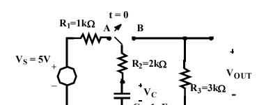
The switch in the circuit moves from A to B at t = 0. Find the output voltage  $V_{OUT}(t)$ .
