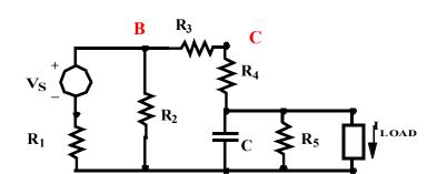
Label the nodes and write a complete set of node equations for determining the node voltages that only contain the node voltages themselves and resistance, capacitance,  $V_S$  and  $I_{Load}$ .
