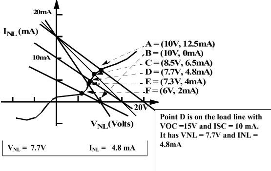
b) Find the power out of the source in the Thevinin equivalent circuit and the fraction of its power that is delivered to the nonlinear load.
