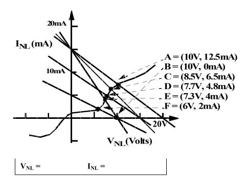
b) Find the power out of the source in the Thevinin equivalent circuit and the fraction of its power that is delivered to the nonlinear load.
