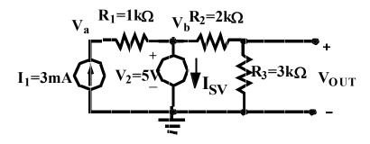
a) For the circuit shown find the Thevinin equivalent circuit looking into the output.
