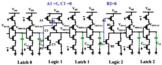
1) System Operation: Assume the clock has a 400 ps high followed by a 200 ps low. Also assume that the input to latch 0 has been low for many clock cycles. Also assume that a latch transition takes 100 ps and that the logic transition for ci5rcuit 1 is 200ps and for circuit 2 is 200 ps. Make a timing diagram for the circuit. That is, first sketch the clock for several cycles and then below it plot the response of each output in the circuit. Sketch the timing after input to latch 0 goes high.
