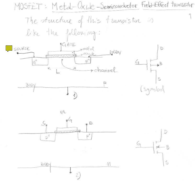
The device in 1) is called m-channel MOSFET and is built on a p substrate. The device in 2) is called p-channel MOSFET and is built on an m substrate. Usually source and body are commected together and this will be the configuration that we will consider.
