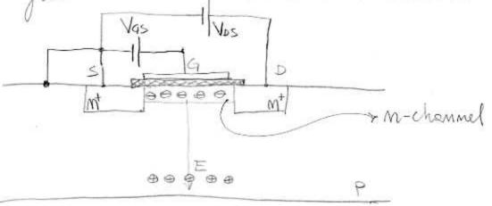
Consider an m-channel Mos where a voltage source is connected between gate and source and drain an source.
