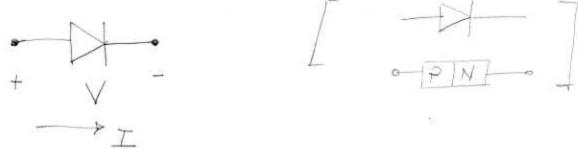
For  $V < V_f$ , I is very small and it V < 0 then  $I \simeq -I_0$  which is a very small reverse arrent.
