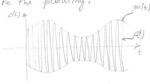
When c(t1) Ve the current will charge the copacitor, when c(t) < Ve the capacitor will be discharged by R.
