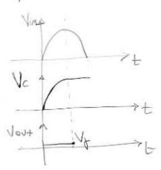
Vout is equal to the voltage across the disole that is by since the disole is ON.
