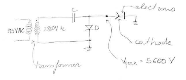
Using the some strategy we can build a full were doubler, a tripler a quadrupler and so on.
