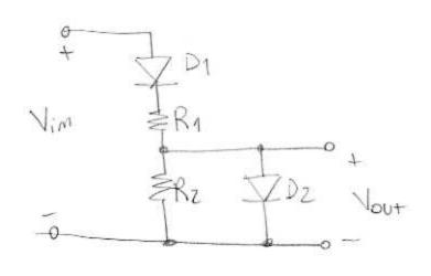
$R_1 = 100 \Omega$   $R_2 = 50 \Omega$   $R_R = 100 M \Omega$   $R_f = 5 \Omega$  $V_g = 0.7$  Since there are two disodes then we have to explore at most 4 states:
