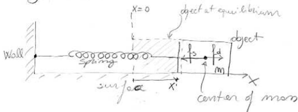
You have probably seen this system before. A spring is attached to a wall. An object of mass  $m$  is attached to the spring. At equilibrium, meaning when the object is at  $x=0$ , the spring force  $f_s$  is equal to 0. If we move the object to the left the spring force increases. If we release the object, then the spring force
