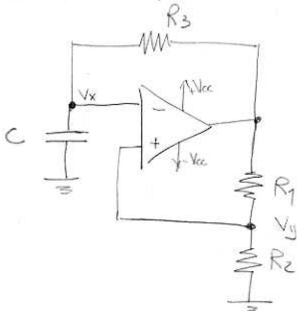
C.1) Consider  $V_x = V_{cc} \frac{R_2}{R_1 + R_2}$  and the output to be  $-V_{cc}$ .
