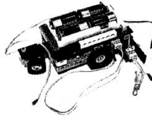
Figure 2.11: TuteBot has motors and batteries wired up and connectorized. The battery case (containing four 1.5 V alkaline C cells) has been mounted above the motors. Wires from the two motors and the battery case are ready to be plugged into the breadboard.
