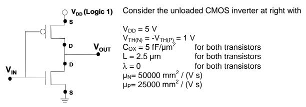
Find a width  $W_N$  for the NMOS transistor channel and width  $W_P$  for the PMOS transistor channel that together will make  $V_M = 2 V$ .
