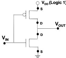
Consider the unloaded CMOS inverter at right with
