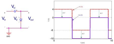
Fig. 11. Reversing the orientation of the diode while keeping the polarity the same.
