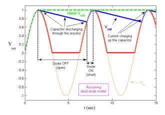
Fig. 21. The plot of the output voltage  $V_{out}$  versus the input voltage  $V_s$ , given the peak detector circuit in Fig. 19 and assuming the ideal diode model. The ideal voltage output is shown in thick dashed lines, when the capacitor is assumed to be nearly infinite.
