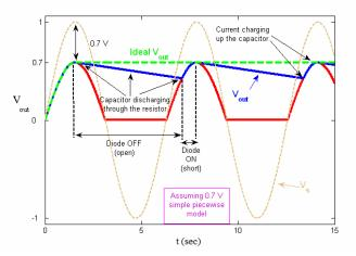
Fig. 22. The plot of the output voltage  $V_{out}$  versus the input voltage  $V_s$ , given the peak detector circuit in Fig. 19 and assuming the 0.7 simple piecewise model. The ideal voltage output is shown in thick dashed lines, when the capacitor is assumed to be nearly infinite.
