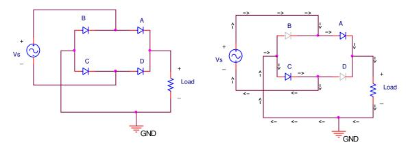
Fig. 17. A full-wave rectifier implemented using a diode bridge model.
