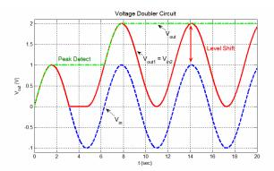
Fig. 24 A plot of the input voltage  $V_{in}$ , the intermediate voltage  $V_{out1}$  or  $V_{in2}$ , and the final voltage output  $V_{out}$ . After the initial waveform, indicated in dash, is shifted upward, the peak detector detects the peak to obtain the final output voltage.
