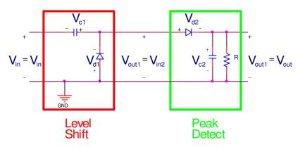
Fig. 23. Voltage doubler circuit. A cascade composition of the level shift circuit with the peak detector. The output of the level shift circuit on the left is passed in as the input to the peak detector circuit on the right.
