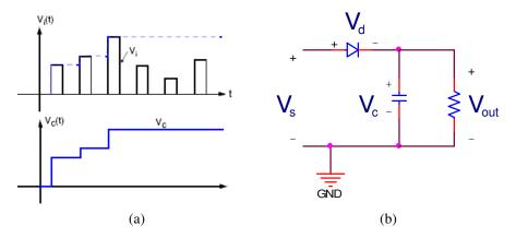
Fig. 20. Peak detection. (a) The top waveform is fed into a peak detector circuit to produce the bottom curve, assuming the capacitance is nearly infinite. (b) Peak detection circuit.
