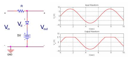
Fig. 6. The  $2^{nd}$  canonical form for analyzing clipper circuit, assuming the simple piecewise 0.7 model. (a) The new circuit with battery added in series with the diode. (b) The plot of the input voltage and the resulting output voltage as a function of time.
