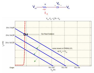
Fig. 2. The load line is shifted in parallel, indicated by the arrow, when the parameter  $V_a$  approaches  $V_{cc}$ , assuming that the resistance is kept at a constant value. The circuit for the particular load line is shown above.
