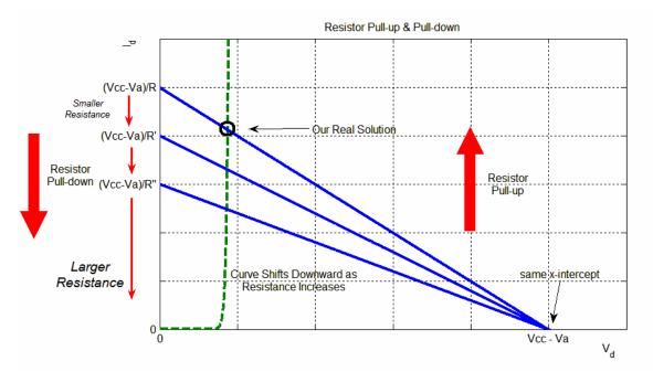
Fig. 3. The load line shifts as we vary the resistance, assuming Vcc and Va as constant. The curve does not shift in parallel because the x-intercept remains the same.
