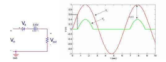
Fig. 15. Adding a 0.6 V battery to the circuit produces the corresponding output signal, shown in green from the input signal, shown in red. Ideal diode model is assumed here.
