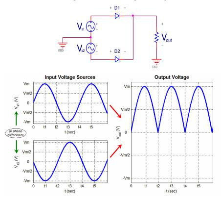
Fig. 16. A full-wave rectifier implemented using two AC sources and two diodes model. The two voltage sources are out of phase, as seen from the left plot.
