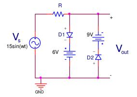
Fig. 8. Clipper circuit diagram.
