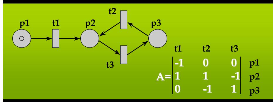
Necessary condition for marking M to be reachable from initial marking M<sub>0</sub>:
