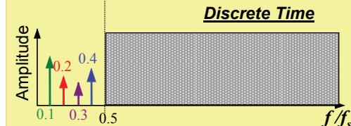
Key point: Signals @  $n f_s \pm f_{max\_signal}$  fold back into band of interest → Aliasing
