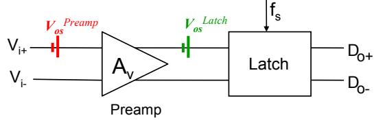
Latch offset attenuated by preamp gain when referred to preamp input.
