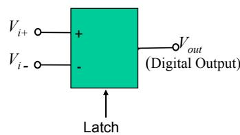
Compares two input voltages at time  $t_x$  & generates a digital output:
