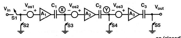
Note: Offset storage capacitors in series with the amplifier outputs
