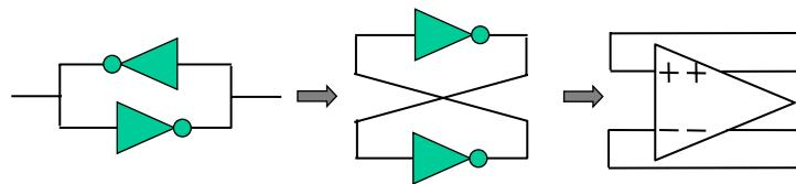
Latch → Amplification + positive feedback
