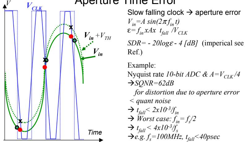
Ref: P. J. Lim and B. A. Wooley, "A high-speed sample-and-hold technique using a Miller hold capacitance," *IEEE Journal of Solid-State Circuits*, vol. 26, pp. 643 - 651, April 1991.
