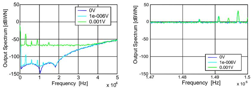
Symmetry of the spectra at  $f_s/2$  and DC confirm that this is AM modulation
