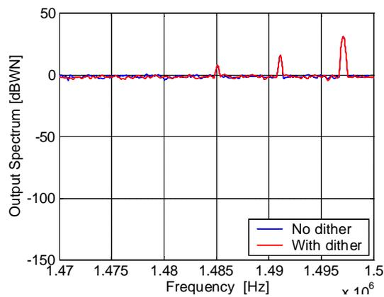
Dither at an amplitude which buries the in-band tones has virtually no effect on tones near  $f_s/2$
