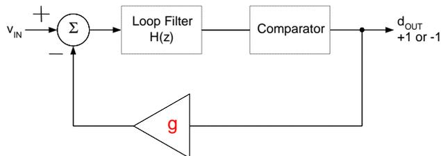
Increasing  $v_{IN}$  &  $g$  by the same factor leaves 1-Bit data unchanged
