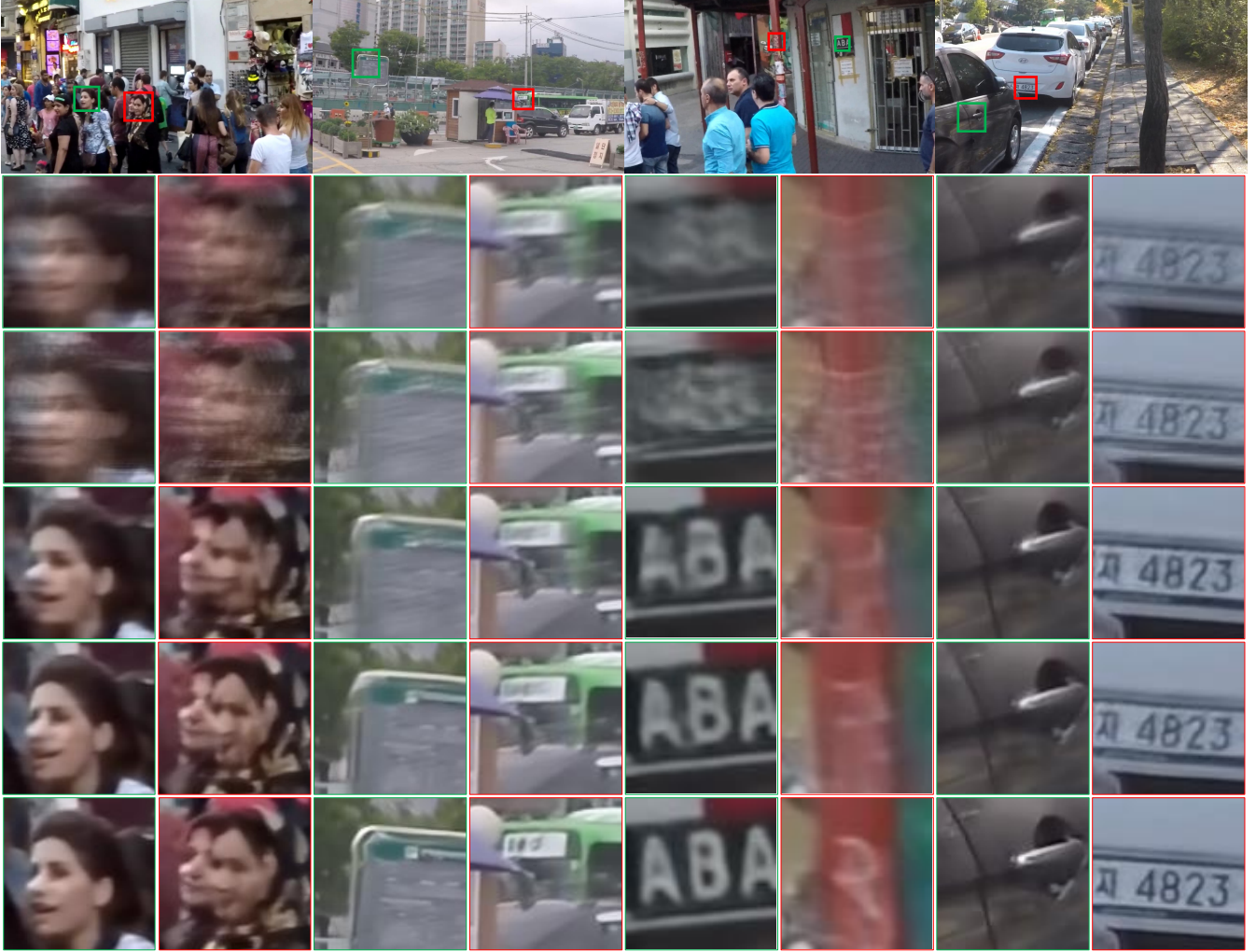
Fig. 4. Visual image quality evaluation on GoPro dataset: from the top to bottom we show blur input and deblur results of DeblurGAN [6], SRN [9], DMPHN [10] and proposed method. We can see that DeblurGAN results are very blur, SRN and DMPHN failed to restore faces, text or details (see billboard or car door).
