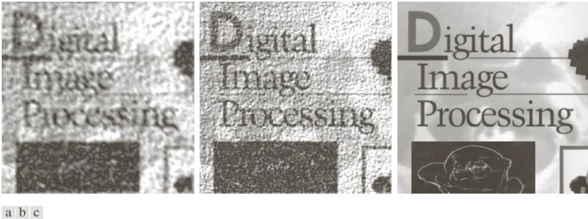
FIGURE 5.30 Results of constrained least squares filtering. Compare (a), (b), and (c) with the Wiener filtering results in Figs. 5.29(c), (f), and (i), respectively.
