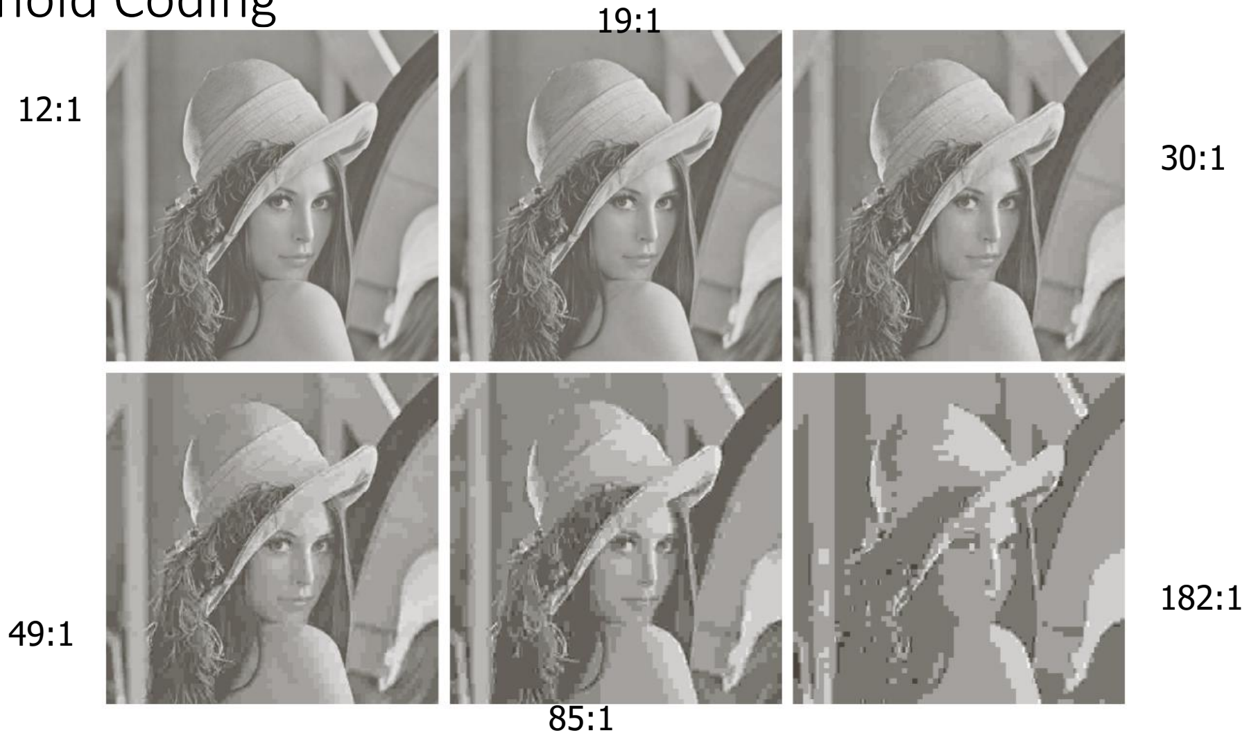
FIGURE 8.31 Approximations of Fig. 8.9(a) using the DCT and normalization array of Fig. 8.30(b): (a) Z , (b) 2Z , (c) 4Z , (d) 8Z , (e) 16Z , and (f) 32Z .
