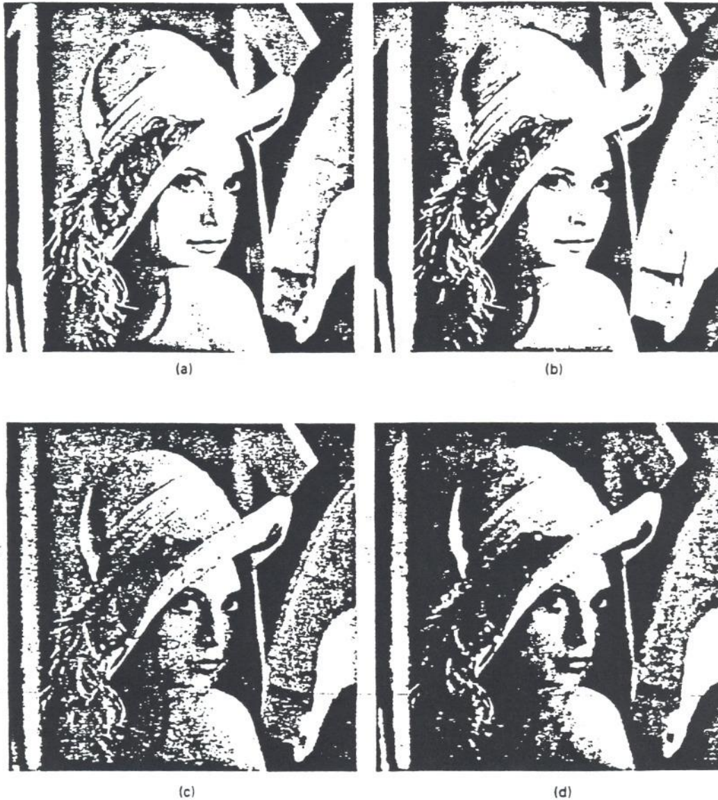
Figure 10.22 Example of quantization noise reduction in PCM image coding. (a) Original image of 512 \times 512 pixels; (b) PCM-coded image at 2 bits/pixel; (c) PCM-coded image at 2 bits/pixel by Robert's pseudonoise technique; (d) PCM-coded image at 2 bits/pixel with quantization noise reduction.
