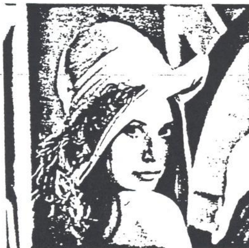
Figure 10.30 Example of differential pulse code modulation (DPCM)-coded image at 3 bits/pixel. Original image used is the image in Figure 10.22(a). NMSE = 2.2%, SNR = 16.6 dB.
