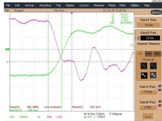
**FIGURE 8.** Measured current and voltage turn-on switching transient.
