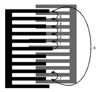
The final example below shows a misalignment of greater than a line and a space. The process is the same as determining any other misalignment except that you need to add the additional line and space width to the offset. This is useful for applications in which the misalignment is very
