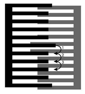
The second example below shows the effect of a misalignment greater than the width of one line but less than the width of a line and space. Notice how there are not enough lines to account for the misalignment. The solution is to wrap around and continue the count. Make sure only to count one of the end lines of the black structure and not both. Since the line count goes upwards, the result shows that the grey structure is shifted up by 0.14 inches.
