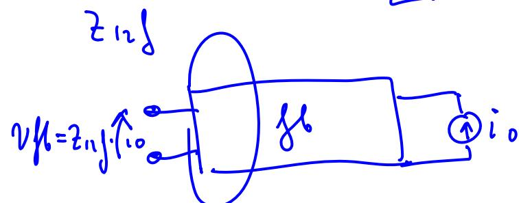
$$z_{11f} = \frac{v_{11f}}{i_o} \quad |_{i_i = 0} = \infty$$
