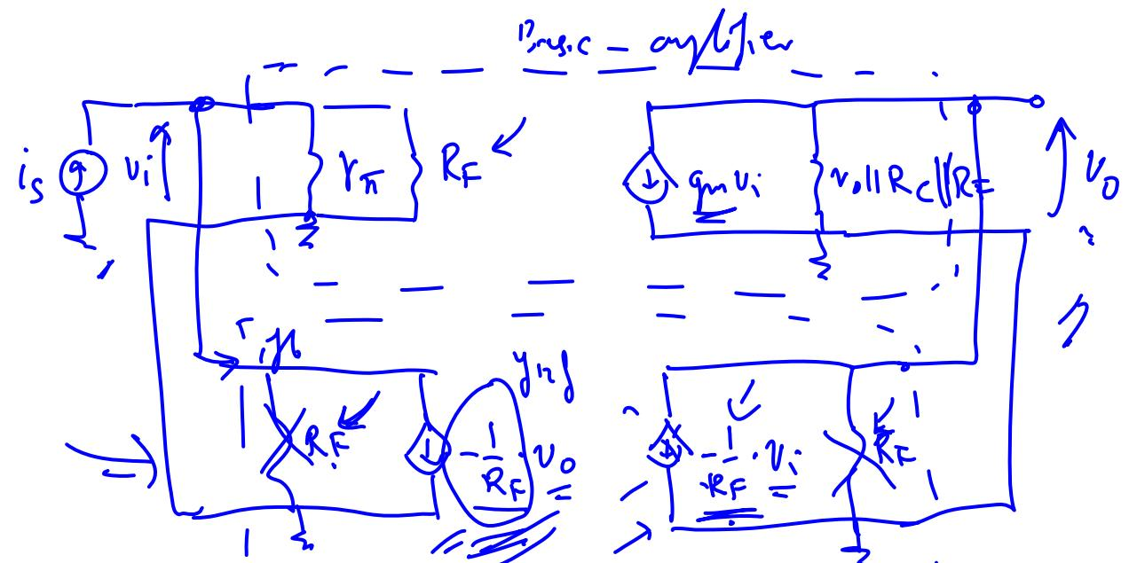
$$\alpha = -\frac{g_m}{r_{\pi} + R_F} \quad \text{Feedback block}$$
