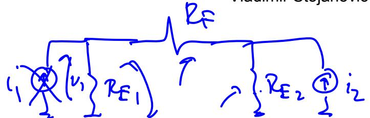
$$z_{22f} = \frac{v_2}{i_2} \Big|_{i_1=0} = R_{E2} \parallel (R_F + R_{E1})$$
