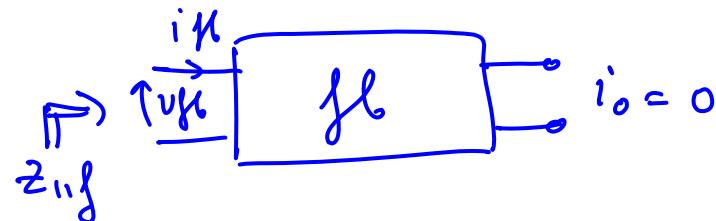
$$z_{11f} = \frac{v_{11f}}{i_1f} = \frac{v_t}{i_t} \quad |_{i_o = 0}$$
