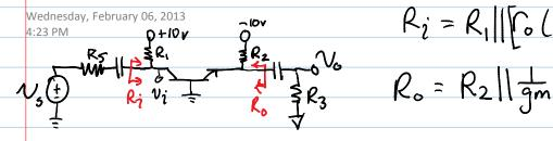
$$R_i = R_1 || [c_0(1 + gm(R_2 || R_3))]$$
