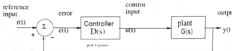
The "Type" of loop refers to the number of poles at  $s = 0$  for the open loop gain,  $DG$ . Type 0 loops have constant steady state error for step response. Type 1 loops have zero steady state error for step response.
