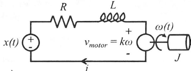
$$a) \quad \int \frac{d\omega}{dt} = k_i i(t) \quad \longleftrightarrow \quad \int s Y(s) = K I(s)$$
