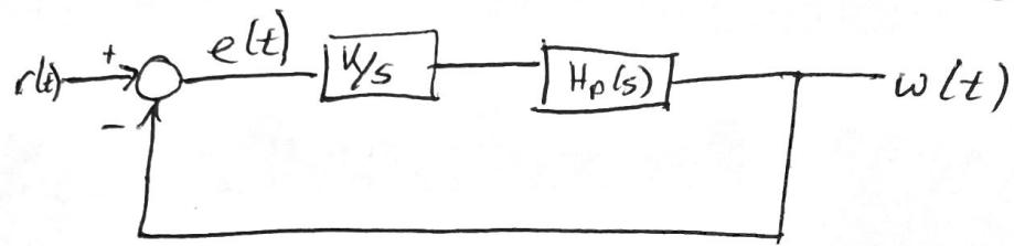
$$E(s) = R(s) - \frac{K}{s} H_p(s) E(s) \quad \lim_{t \rightarrow \infty} e(t) = \lim_{s \rightarrow 0} s E(s)$$
