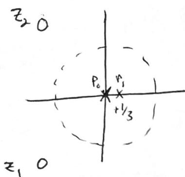
$$\begin{array}{ll} z_2 @ -\frac{3}{2}e^{-j\pi/4} & P_0 @ \text{zero} \\ z_1 @ -\frac{3}{2}e^{j\pi/4} & P_1 @ +\frac{1}{3} \end{array}$$
