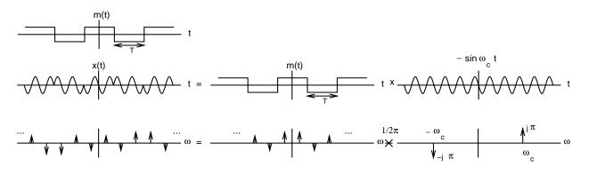
Figure 1: Frequency analysis of PM square wave modulation.
