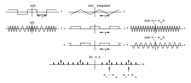
Figure 2: Frequency analysis of FM square wave modulation.
