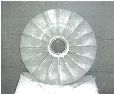
Figure 3. Turbine compressor, front view. [2]
