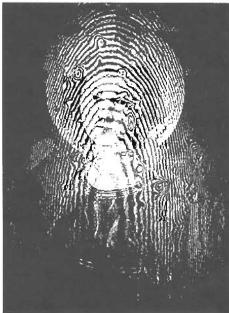
Figure 11. Holographic interferogram made using thermal-drift method, revealing detachments. [4]
